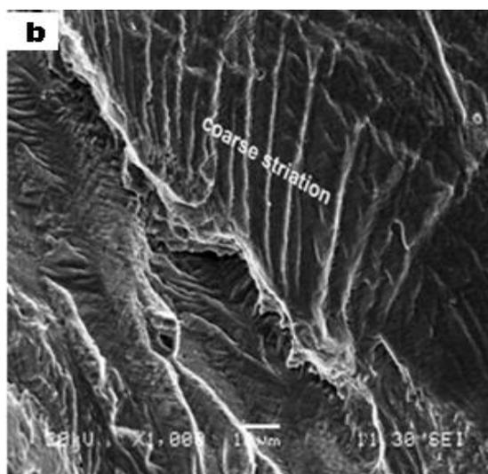
Figure 7: INCONEL601 specimen show dimples and larger striations at 650,000 cycles, at low (a) and high magnification (b).
