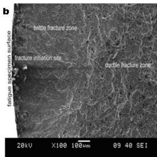
Figure 3: INCONEL601 specimen fracture surface shows brittle and ductile zones, (a) Fracture at 250,000 cycles, and (b) at 350,000 cycles.
