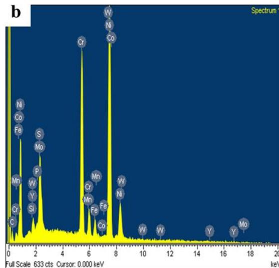
Figure1: INCONEL601 specimen, (a) SEI of polished specimen showing triangular carbides at the grain boundaries and slip bands, and (b) EDS X-ray spectra.
