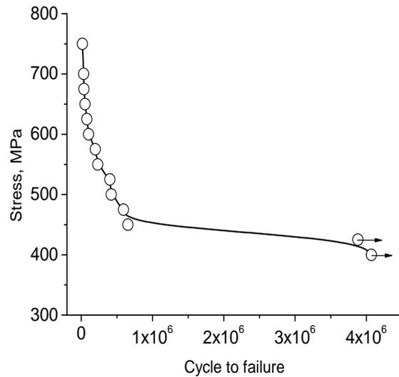
Figure 2: S-N curve of INCONEL601 showing that no fracture occurs below 500MPa.
