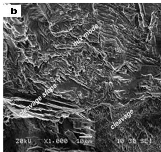
Figure 4: INCONEL601 specimen shows cleavage and mixed mode at 400,000 cycles, at low and high magnification (a), and (b) respectively.
