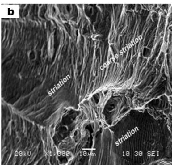
Figure 6: INCONEL601 specimen shows dimples and striation at 550,000, at low (a) and high magnification (b).
